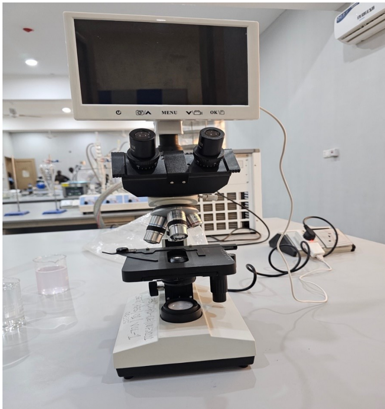
Name: Digital Trinocular Microscope with built-in-LCD Screen AmScope brand (XSZ-107BN model)
