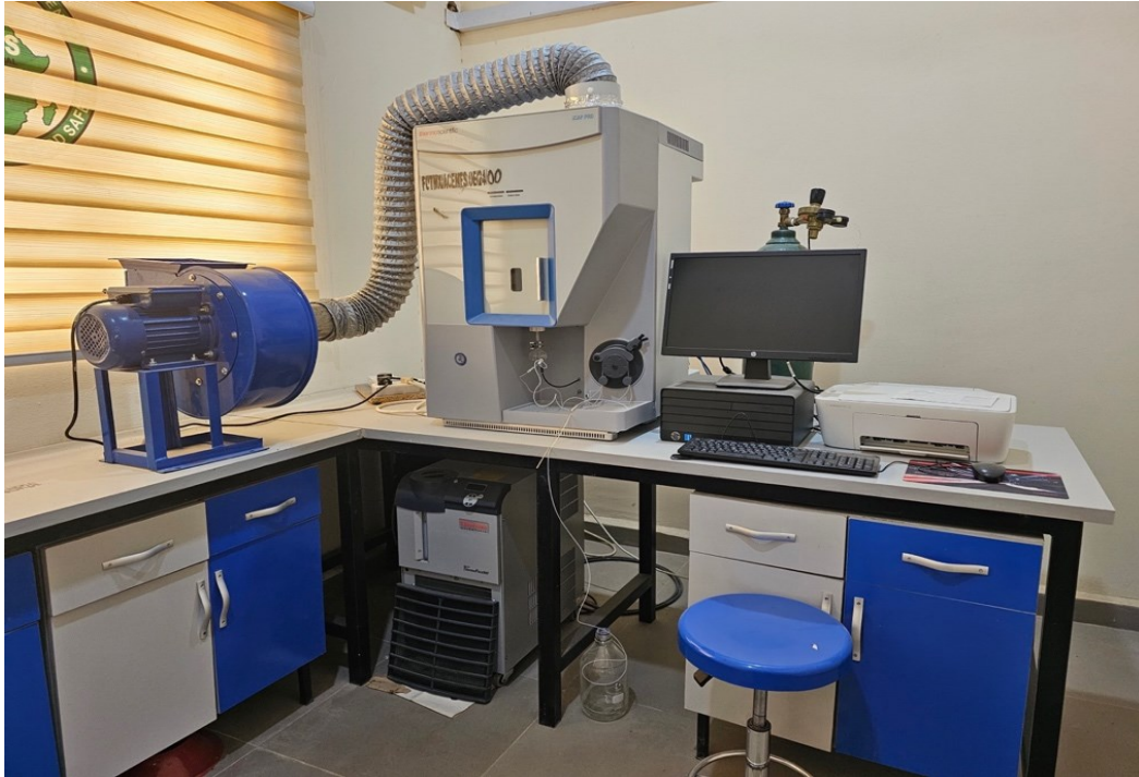
Name: Thermo Scientific iCAP PRO Series Inductively Coupled Plasma-Optical Emission Spectrometry (ICP OES) Systems (Thermo Fisher Scientific)
