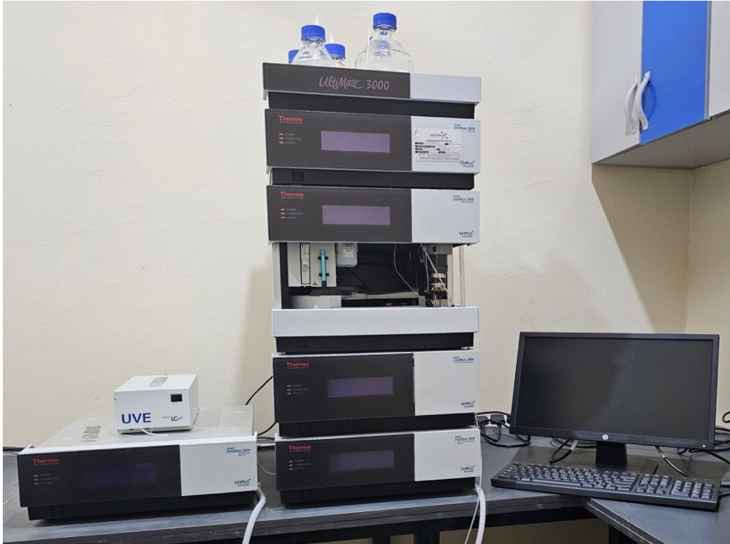
Name: Thermo Scientific Dionex UltiMate 3000 HPLC System with DAD-3000RS Diode Array Detector
