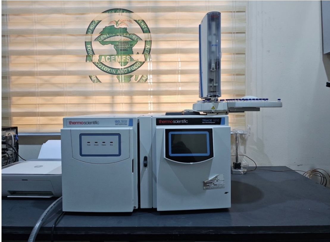
Name: Thermo Scientific ISQ 7610 Gas Chromatography Mass Spectrometry (GC-MS) System, coupled with a TRACE 1610 Gas Chromatograph
