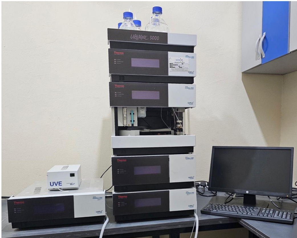
Name: Thermo Scientific Dionex UltiMate 3000 HPLC System with DAD-3000RS Diode Array Detector
